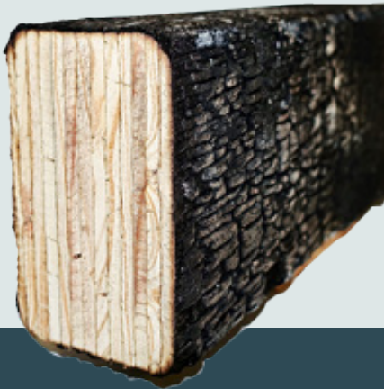
Fig. 1 Charred LVL beam
