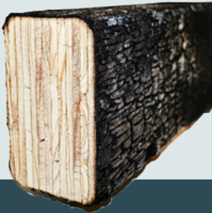
Fig. 1 Charred LVL beam
