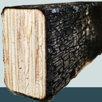
Fig. 1 Charred LVL beam
